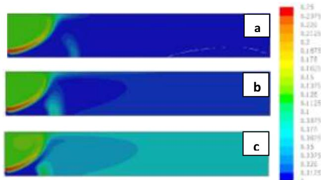
Fig.14 Oxygen mass fraction maps (a) T.L. = 44 kW, (b) T.L. = 55 kW and (c) T.L. = 75 kW
